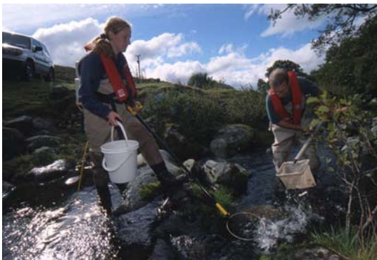
Rapid semi-quantitative electrofishing in action! It only requires two operatives, battery driven backpack equipment and no stop nets. Photo courtesy of A.Tryner and the Countryside Agency.
